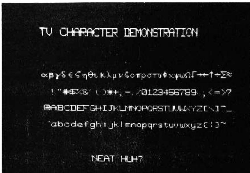
all 7 dots into its internal memory, and then outputs these dots one at a time for serial transmission to a TV set. For more information on TV character generators, I would suggest reading an excellent article by Don Lancaster in June 1974 *Radio Electronics* [pages 48-52], or the June 1976 *BYTE* magazine article by C W Gantt [page 16].
