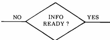
Lines with arrows may be used to interconnect the three types of symbols presented. In this way, the symbols may be connected to form readily understood FLOW CHARTS of operations that are to occur in a program and to show how various operations relate to each other. Flow charts are extremely valuable references when developing programs as well as when one wants to update or expand a program and needs to quickly review the operation of the program of specific interest.
