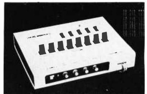
We received this picture of a new Model 100A Logic Analyzer, produced by Paratronics Inc, 150 Tait Av, Los Gatos CA 95030, and seen in some detail in *Popular Electronics*, February 1977. This unit is available in a complete kit for \$198.50, along with a 100 page assembly and applications manual.
