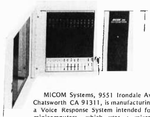
MICOM Systems, 9551 Irondale Av, Chatsworth CA 91311, is manufacturing a Voice Response System intended for minicomputers, which uses a micro-processor as a control element. The press release describes a system which can accept Touch-Tone encoded inputs and give digitally generated synthetic voice outputs. This system, which is definitely oriented toward commercial systems markets, has prices beginning at \$500.■
