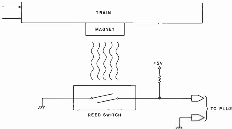
Figure 4: Reed switch circuitry used to send feedback information to the microcomputer. When a train passes by, the magnetic field causes the switch to close, pulling the signal line down to ground potential; this sends a signal back to the interface (and finally to the computer) that a train is passing.
