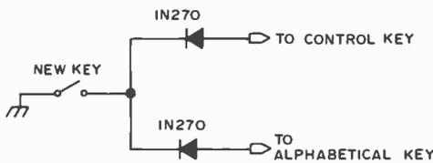
Figure 2: Simple circuit to add control keys to a keyboard. The new key is wired to both the control key and the alphabetical key. The diodes are needed to isolate the keys from each other.
