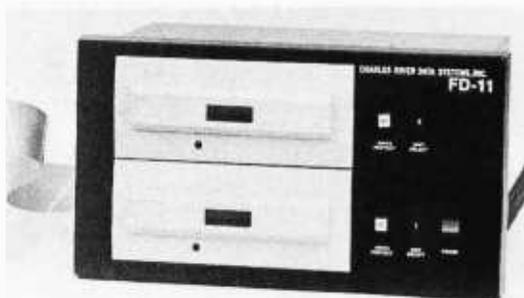
software and media compatible with the DEC RX11 products. It includes write protect switches, unit select switches, up to four drives with one unit load on the DEC Unibus, PROM self-diagnostic programs and bootstrap loader. Track to track access time is 6 ms. Single quantity price of the drive and DEC compatible controller is \$2750. ■
