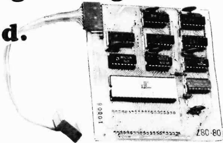
**DUTRONICS**<sup>®</sup> a leader in low cost, low power ram boards has just announced it's Z 80 - 80 piggy back card. This plug - in board enables you to use your existing IMSAI, ALTAIR CPU card and upgrade your system to a Z - 80.
