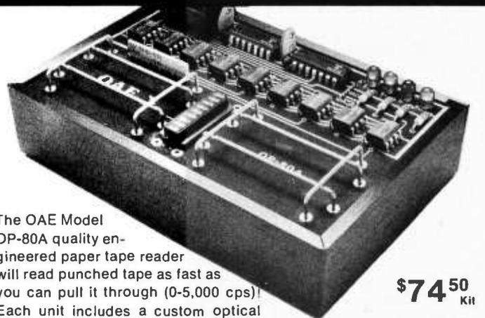
The OAE Model OP-80A quality engineered paper tape reader will read punched tape as fast as you can pull it through (0-5,000 cps)! Each unit includes a custom optical sensor array, high speed data buffers, and all required handshake logic to interface with any microprocessor parallel I/O port. Check our specs. AT OAE WE MAKE QUALITY AFFORDABLE!
