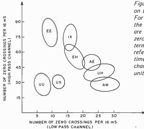
Figure 3: Vowel formants on the zero crossing plane. For comparison purposes the formants in figure 1 are plotted here on the zero crossing plane. The term "zero crossing rate" refers to the number of times that the voice signal changes its polarity per unit time (see figure 4a).
