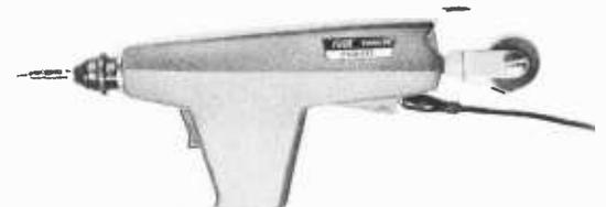
110 VAC powered wrapping tool. This \$80 tool will accept the P180 Slit-N-Wrap tool bit, or a standard wire wrapping attachment in the form of the P160-2A wrapping bit. While Slit-N-Wrap can be done by hand, it becomes much more convenient when it is powered as with this tool. (Because the Slit-N-Wrap technique requires no stripping of wire, it tends to be somewhat faster than standard wire wrap as a matter of course,
