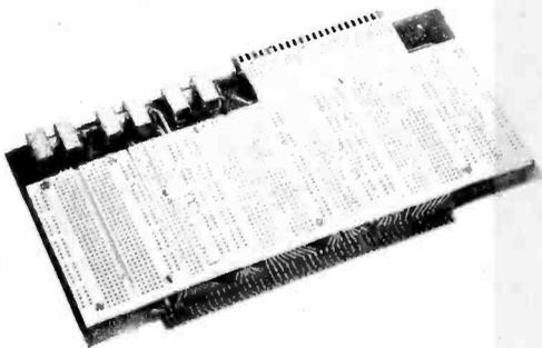
This breadboarding card makes it especially convenient to add experimental circuitry to an Altair (S-100) bus
