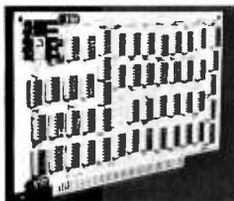
Altair/IMSAI compatible board catches program bugs and provides timing for real-time applications.
