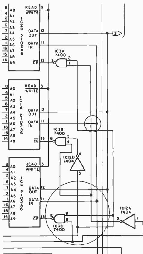
The drafting bug has bitten BYTE. The accompanying figure detail (taken from figure 1a of David Allen's article, "A Floppy Disk Interface," January 1978 BYTE, page 61, right-hand side) contains a number of drafting errors inadvertently included during the production of the article. The corrections are circled. In addition, IC18c, a three input AND gate, was incorrectly drawn as a NAND gate, and the A1 and A2
