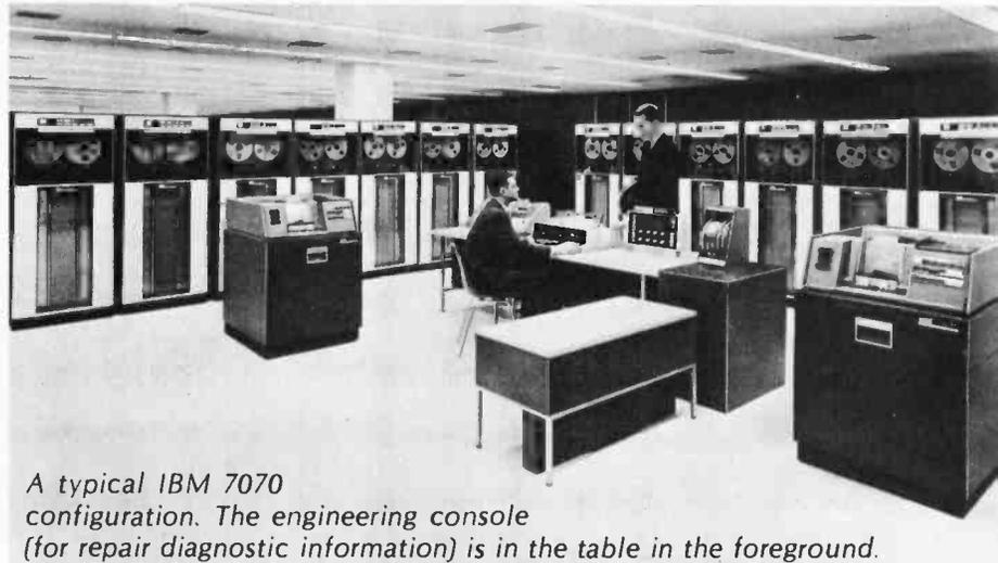
*A typical IBM 7070 configuration. The engineering console (for repair diagnostic information) is in the table in the foreground.*
