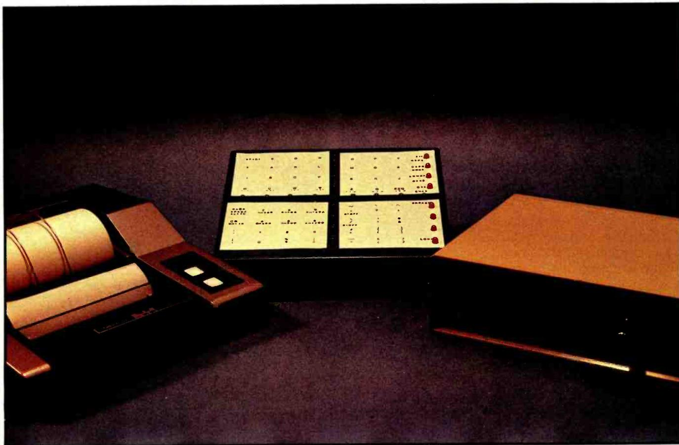
**Photo 1:** The H-Com scanning communicator, a kind of keyboard simulator, can be used to send text directly to a printer, such as the Radio Shack CGP-115 shown here, or to a text-to-speech synthesizer, such as the Intex Talker, in this fully configured system. Using the serial-output commands and phrase mode, the H-Com can transmit words and sentences from a prestored vocabulary.
