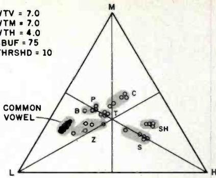
**Figure 4:** An example of consonant plots based on the use of voice, mid, and high bands. Sounds were consonant-vowel pairs with a common vowel (the dark cluster at the left). CBUF refers to the number of consonant samples taken within each utterance.
