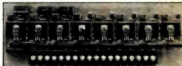
**120 VAC CONTROL.** This board has eight optically isolated triac switches. Each switch can control 200 watts. It connects via a 16 pin ribbon cable to a parallel output port. Screw terminals are provided for 120 vac connection. Part number 82-332. \$119.95.
