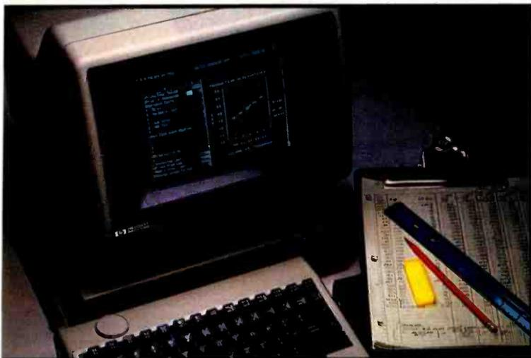
**Photo 3:** The Model 16, shown here with a dual 3 1/2-inch floppy-disk drive, takes up a small amount of desk space. Note the "knob," a one-dimensional track ball, on the upper-left corner of the keyboard.
