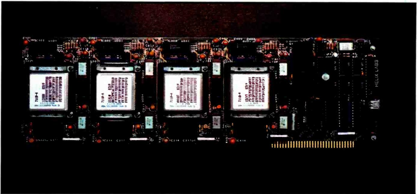
**Photo 4:** The 4-megabit Helix bubble-memory board plugs into an IBM Personal Computer slot for quiet, nonvolatile mass storage. The Helix PCBMs is switch-selectable (on-board ROM BIOS bootstraps DOS from the bubble or floppy disk) and is configured as a fixed disk.
