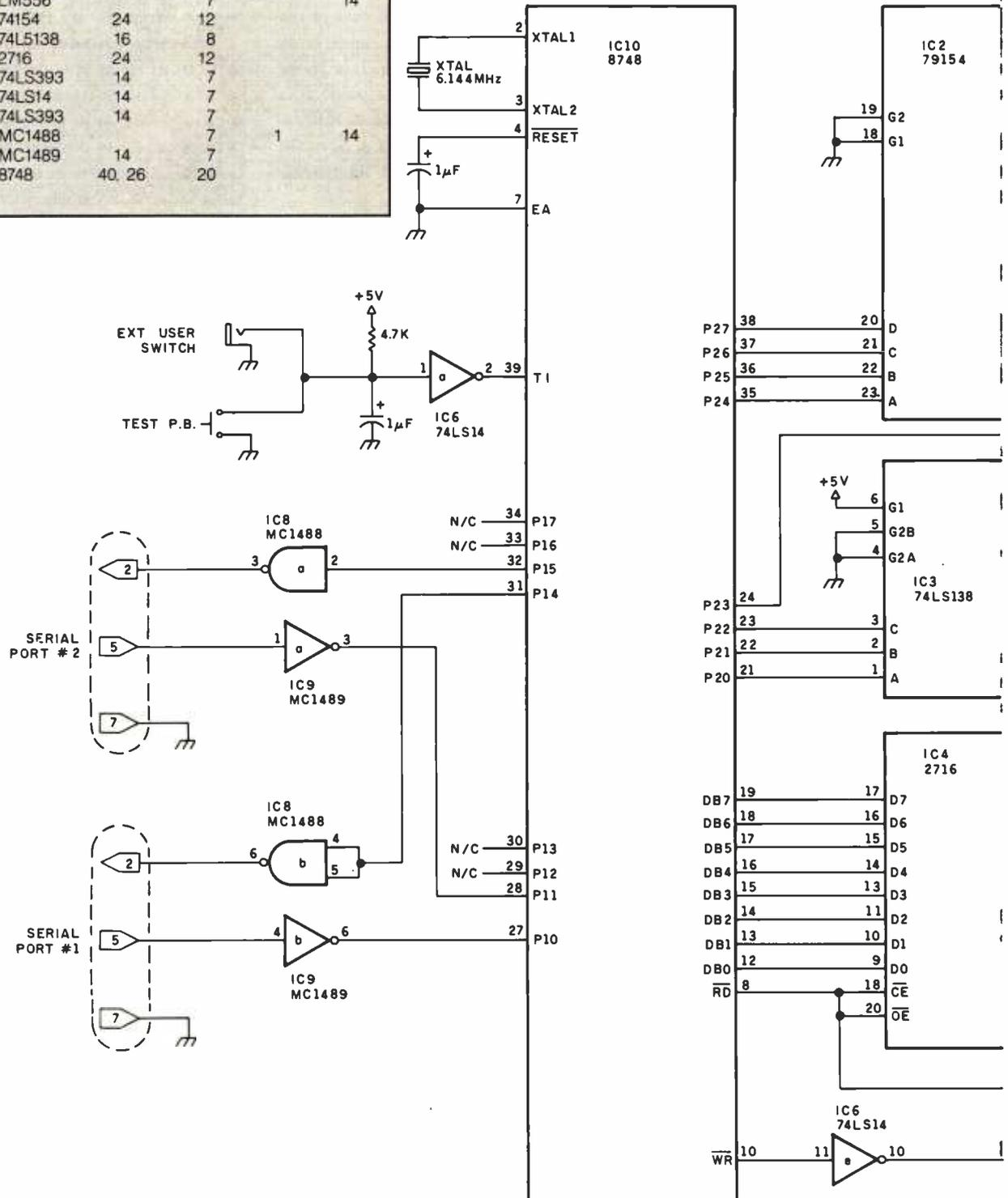
**Figure 2:** The schematic diagram of the H-Com. The external EPROM (IC4, a 2716) is used for storage of mnemonically keyed phrases; addresses for the EPROM are generated by the two binary counters IC6 and IC7.
