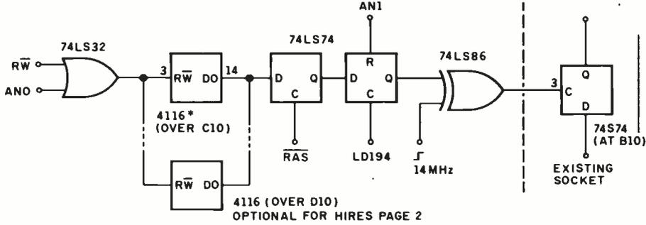
\*ALL CONNECTIONS TO THIS 4116 ARE IN PARALLEL WITH THE EXISTING 4116 AT C10 EXCEPT FOR RW AND DO.
