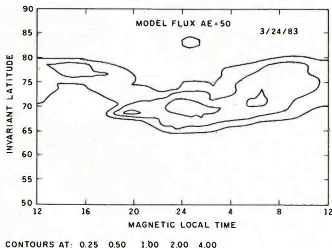
**Figure 1:** This contour plot, based on an array of 960 observations (24 by 40), was made using Condot. The program was run on a Tektronix 4052, and the output was sent to a Tektronix 4662 pen plotter. It took about 10 minutes to generate the plot.
