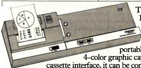
The optional CE-150 Color Graphic Printer/Cassette Interface not only gives the system portable printing but also 4-color graphic capabilities. And as a cassette interface, it can be connected with up to two cassette tape recorders—one for storage and one for recall.
