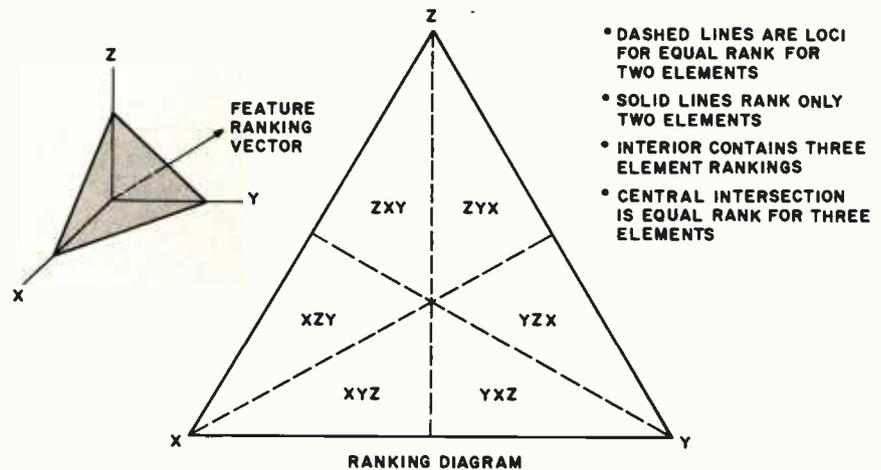
Figure 3: This figure is a ranking diagram, a convenient means of conveying the relative level of three variables. You can thus look at figure 1 and determine that the *i* vowel has its strongest component in the high band and its weakest in the mid band.
