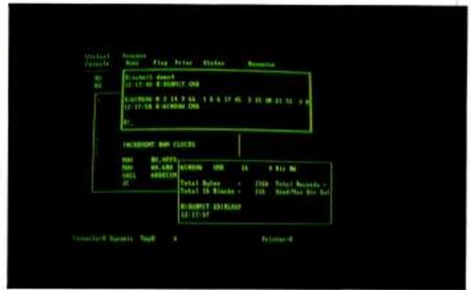
Photo 1: Two examples of dynamic windows, which allow a user to work and monitor several other consoles at the same time.
