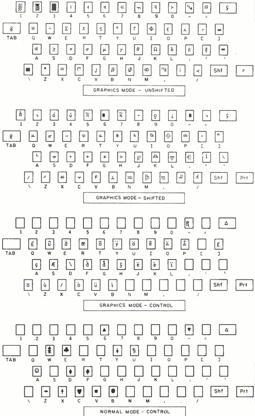
Figure 6: Graphics can be generated in four different Glyphs keyboard modes.
