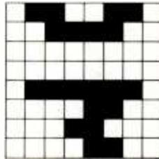
Figure 2: Redefined characters for use with the ANTIC 3 mode. The lowercase g (2a) will have a descending tail, and the 3 (2b) can be used as a subscript character.
