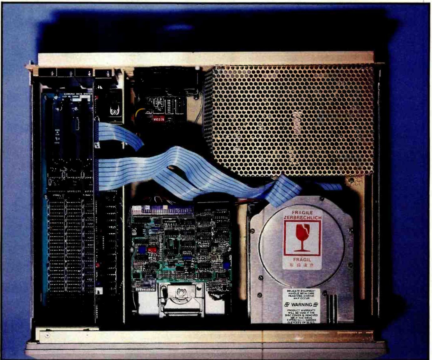
**Photo 8:** Inside the Corona. A Seagate hard-disk drive is on the lower right and the expansion slots are on the left. One of the slots is taken up by the hard-disk controller. The power supply is on the upper right.
