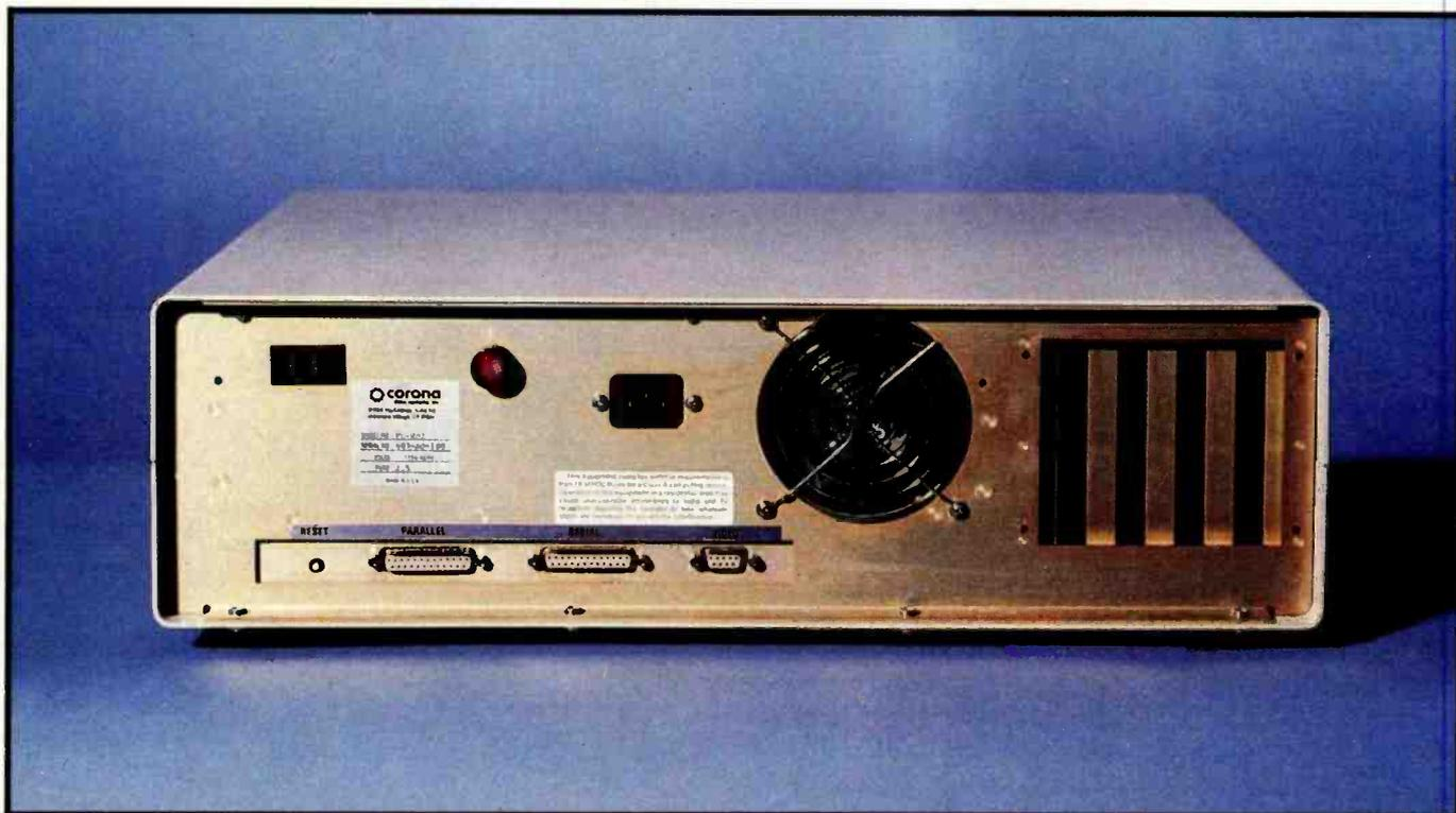
**Photo 7:** The back panel of the Corona. Note the Reset switch on the left, the parallel-printer port, the serial port, the video-display port, and the openings for the expansion cards.
