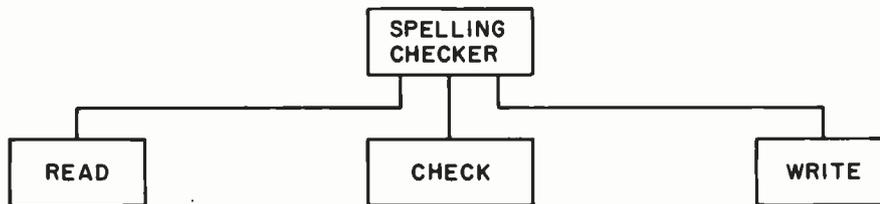
**Figure 2:** This diagram is an example of a "source, transform, sink" problem structure. The main module calls the three subordinates in order from left to right, repeating the process until the input is exhausted.
