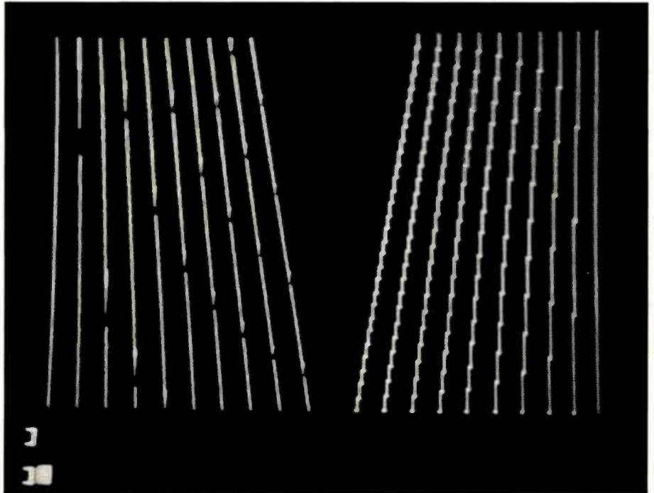
Photo 3: A black-and-white example, created using phase-shifted plotting. The left side was drawn using selected HCOLOR= values; the right half was plotted with the standard HCOLOR=3 (white).
