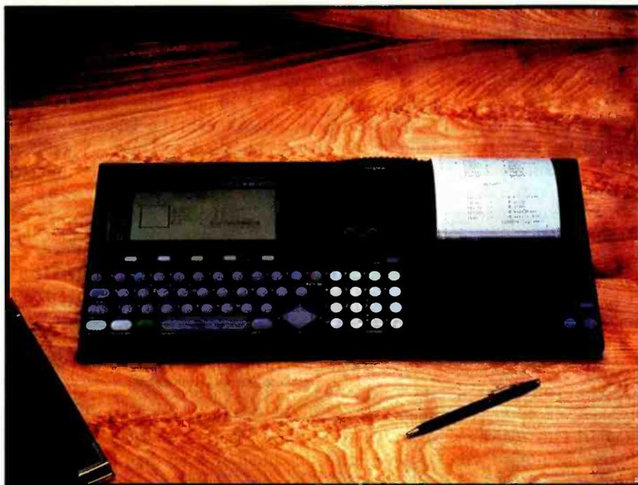
**Photo 2:** The Workslate options. The battery-powered plotter can form 40 to 80 characters in four colors on a line or print them sideways for extra-wide spreadsheets. The Metric converter template on the screen comes on the Travel Taskware tape.
