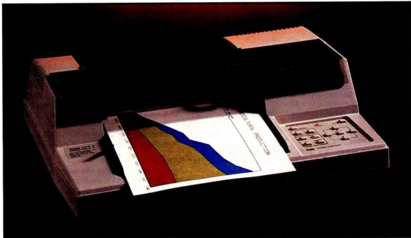
**Photo 4:** The HP 7470A two-pen plotter. This plotter comes with either an HP-IB connector for use with the Series 200 Model 16, or an RS-232C connector. It uses 8½- by 11-inch paper, and more than two colors can be plotted by manually changing the pens. The list price for this plotter has been recently reduced to \$1095.
