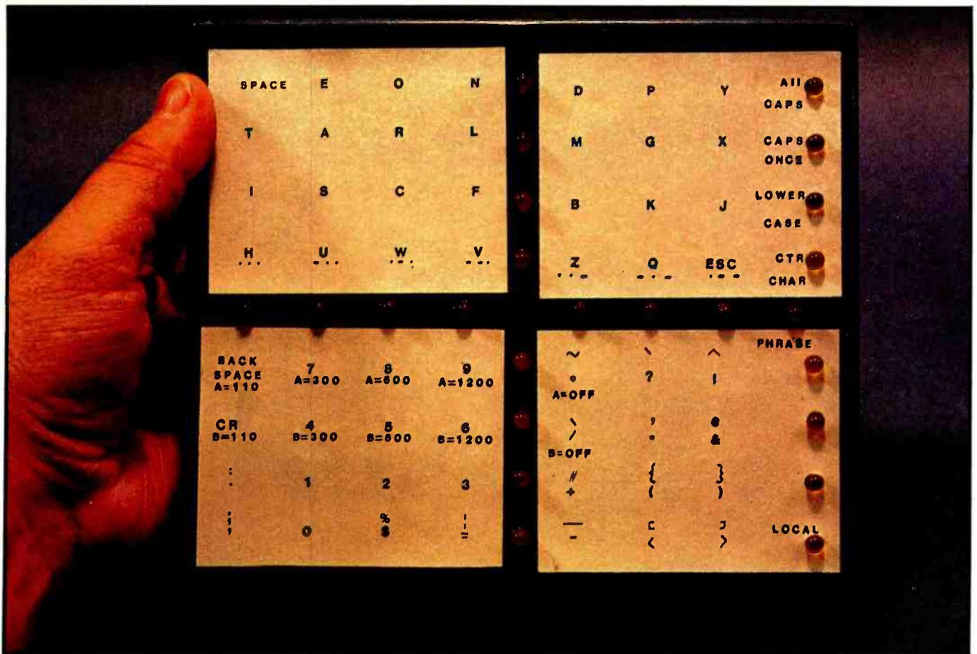
**Photo 3:** The H-Com's character display contains 8 rows and 8 columns of characters and control functions, numbered from top to bottom and from left to right. The intersecting lines of red LEDs are used in scanning the row and column positions, while the yellow LEDs along the right edge indicate which mode is in use.
