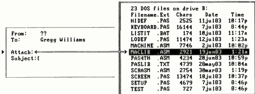
Figure 8: When mail is being sent between PCs, disk files can be sent along as attachments.
