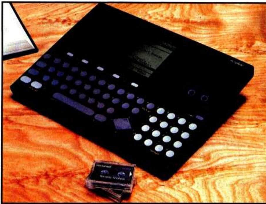
**Photo 3:** The Workslate's calendar is resident in ROM and can be assigned to any Worksheet with the Time function key. The user-modifiable template has formulas for a two-week calendar. Reminder alarms can be set for any appointment. Battery power keeps RAM memory active, and a backup battery provides an extra two months of memory protection.
