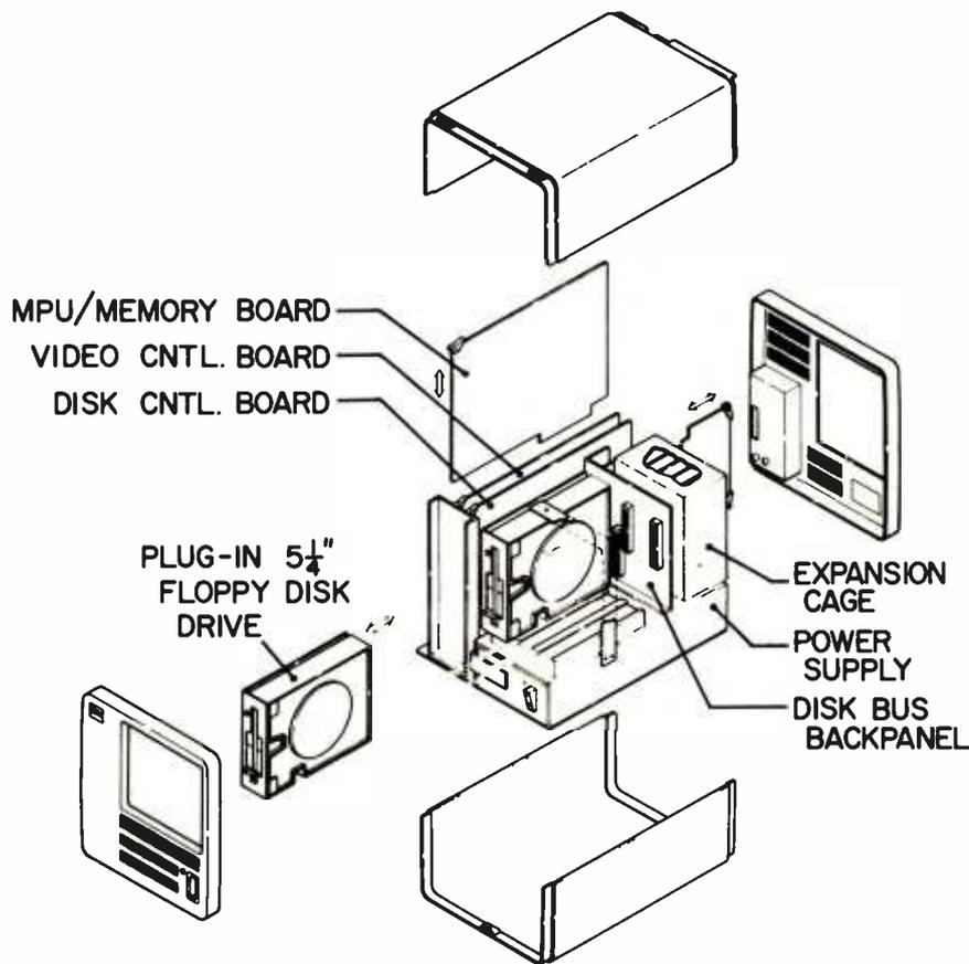
**Figure 1:** Exploded view of the IBM 5550 system unit. Five option boards may be installed in the expansion cage. A hard-disk drive may be substituted for the two right-most floppy-disk drives. (Figure courtesy of IBM.)
