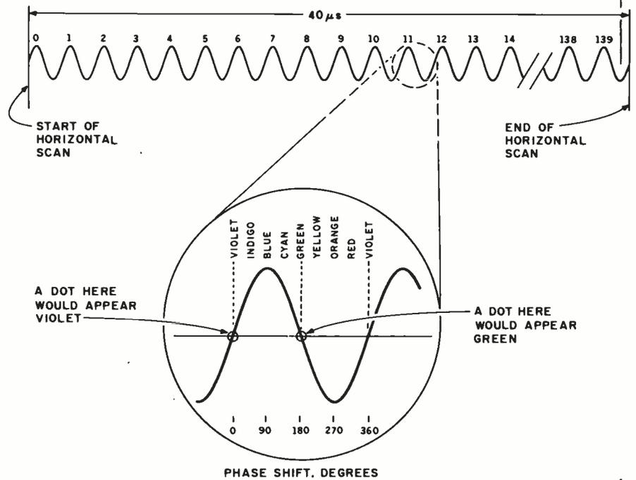
Figure 2: A representation of the phase relationship of a pixel.
