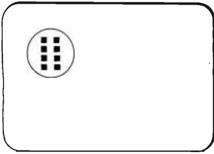
**Figure 1:** A typical arrangement of the contact points of an active memory card. Relatively few (six to eight) contacts are needed because the data is transmitted serially. See the Flonic security card in photo 1.
