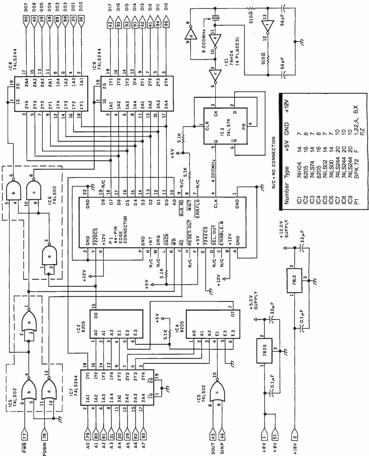
**Figure 2:** A schematic of an S-100 interface and clock circuit for the BPK 72. The kit is used as though it were a single component. Only the edge connector is shown in this figure. The schematic placement of the edge-connector pins matches that of the actual physical component. The completed project functions as either a disk emulator or a cache memory system.
