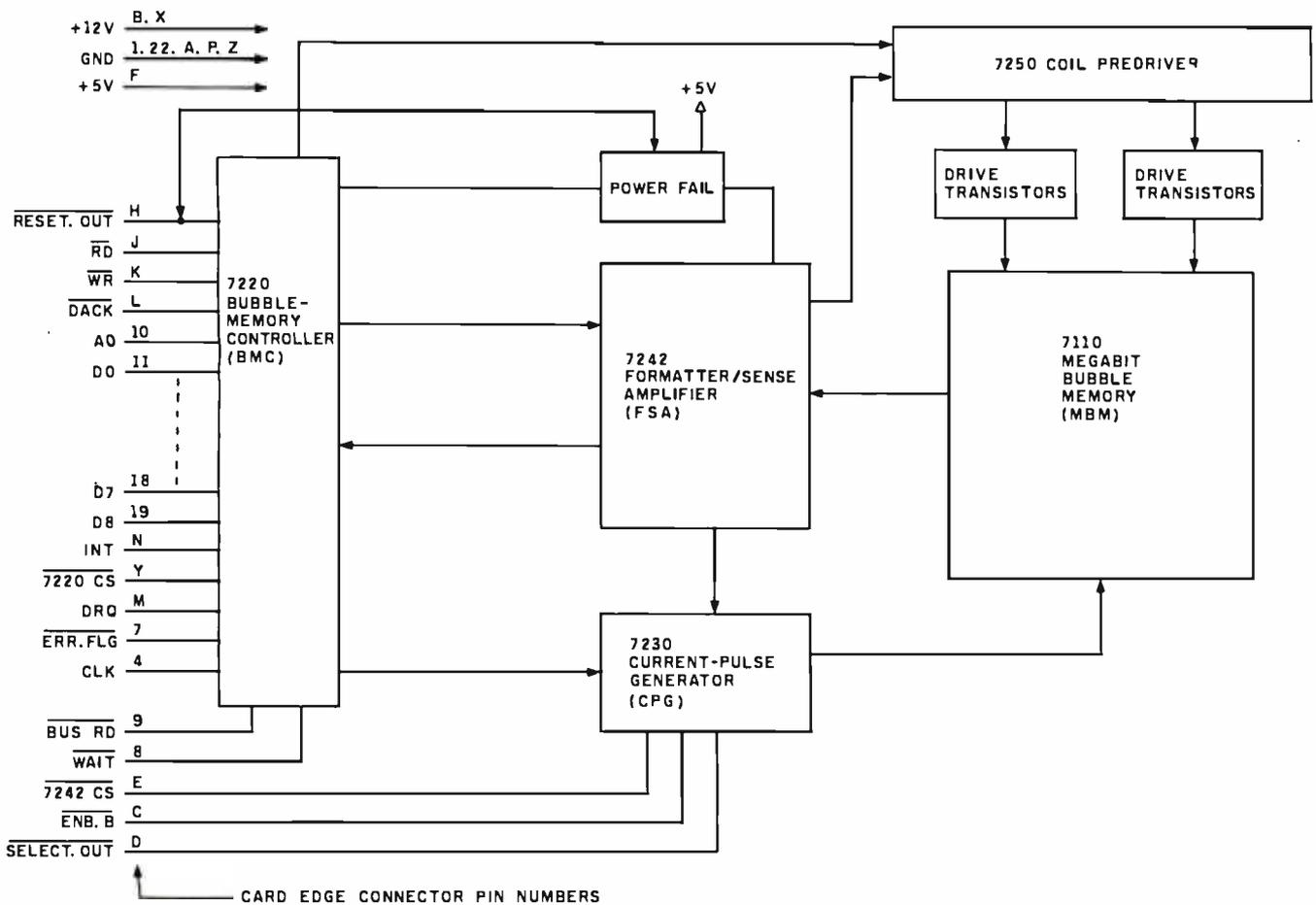
Figure 1: A block diagram of the BPK 72 Bubble-Memory Prototyping Kit.
