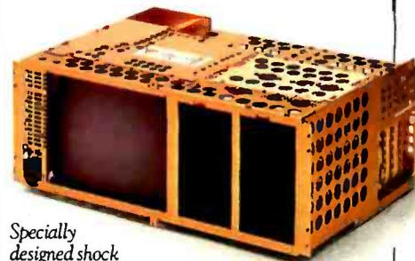
*Specially designed shock isolation system protects the fixed disk from jolts.*
