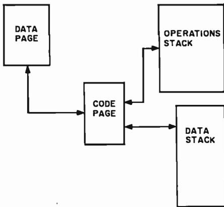
**Figure 1:** The interacting resources of the Reason software bus. Each software component on the bus has a code for the program's source code, a data page for variable storage, and operations and data stacks, the "scratchpads" for program operation.
