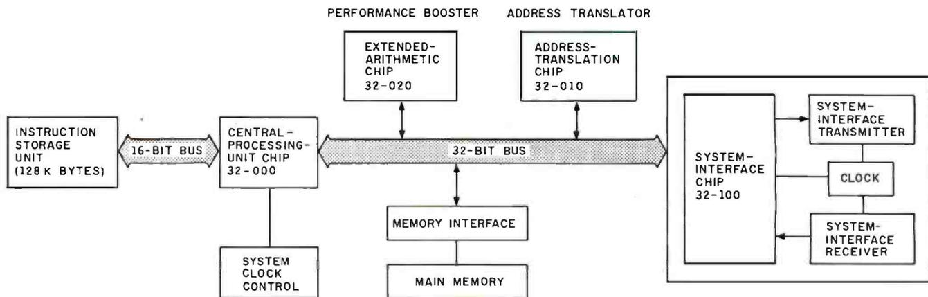
Figure 3: A configuration of the NCR/32 System.
