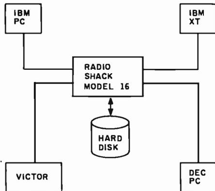
**Figure 2:** Each microcomputer runs a version of a Datanet. Datanet masks the differences between each node microprocessor and the network environment. Microcomputers in the network share data as well as execute programs interactively.
