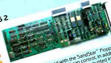
This System is equipped with the SandStar™ Floppy Drive Controller Card. The Card can control, in addition to the Hard Disc Drive, two floppy drives mounted inside your PC and optionally two additional 5 1/4" or 8" drives mounted externally. This leaves three system slots for other expansion boards.
