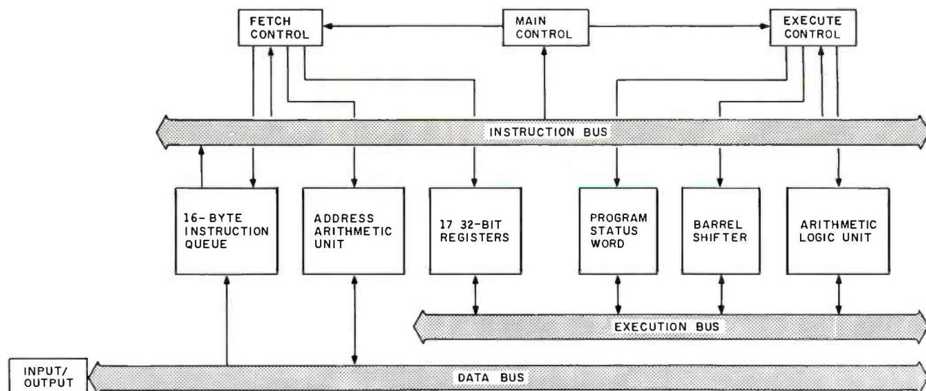
Figure 4: A block diagram of Western Electric's WE32000.
