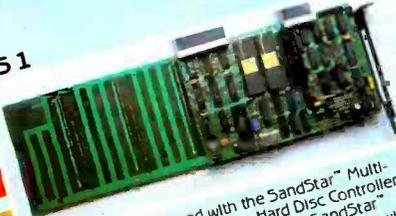
This System is equipped with the SandStar™ Multi-function card. In addition to the Hard Disc Controller Module, you can add up to three other SandStar™ Modules while using only one card slot. The following modules are available: Serial Port, Parallel Port, Clock Calendar, Game Adaptor, SASI Host Adaptor and Prototyping Module.
