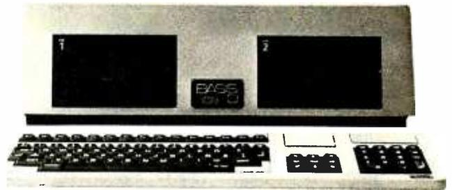
Photo 1: The Basis ("Bah-zis") 108 is a microcomputer, configured like an Apple II, with Z80 and 6502 microprocessors and 128K bytes of RAM. The 108 comes with two Basis disk drives. The earlier model (shown here) has Micro-Sci drives. The keyboard provides all the features required of a business system.
