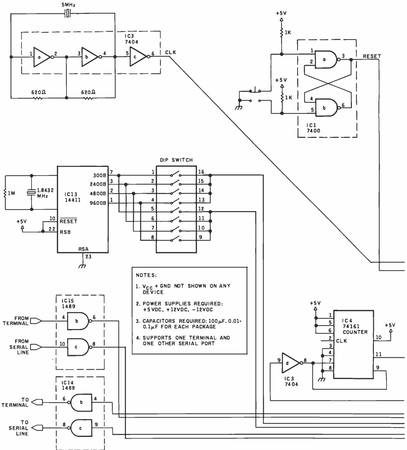
Figure 1: The VU68K schematic.
