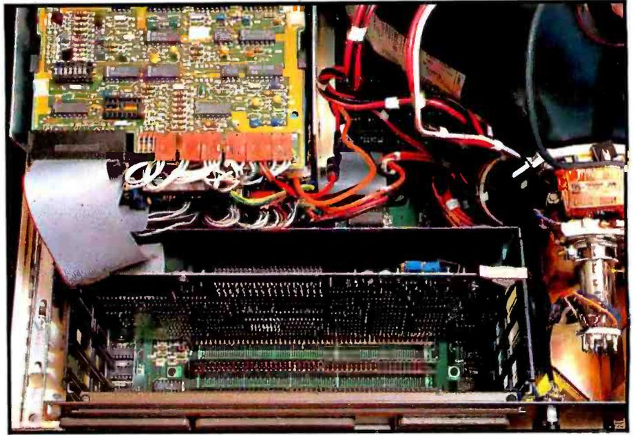
**Photo 5:** Inside the Z-100. The S-100 bus sits behind the disk drives and disk-drive controller (upper left) and the display (upper right). Access to this bus is very simple. The top cover of the machine can be easily removed, without unfastening any screws.
