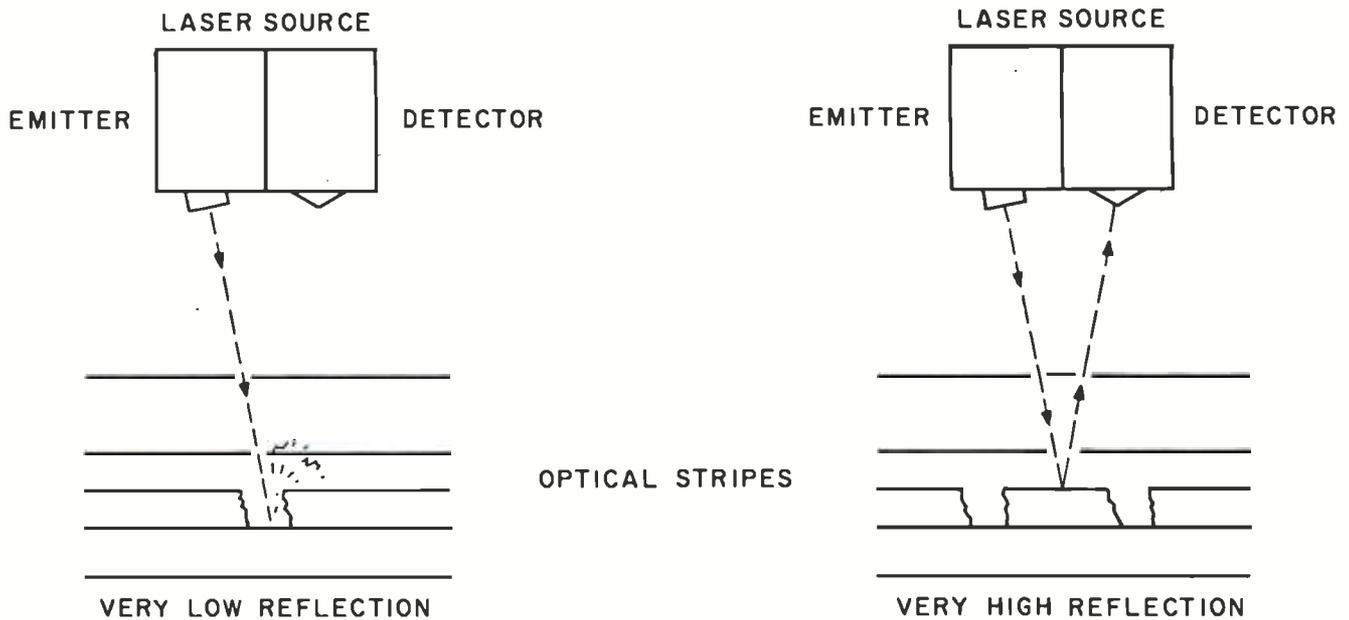
**Figure 5:** The process of reading data encoded on an optical stripe. On the left, the laser beam encounters a hole written in the reflective layer so no light reaches the detector. On the right, the beam is reflected to the detector from an undisturbed section of the reflective layer.
