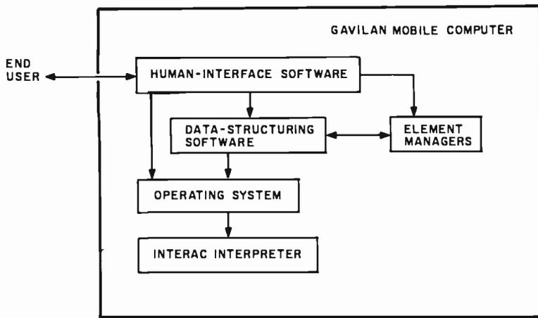
**Figure 2:** The structure of the Gavilan computer's software, showing the main software components and their relation to one another.
