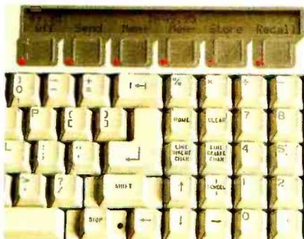
The unique MicroScreen™ serves as a calendar/clock, a built-in calculator, and a labelling device for special touch-sensitive keys.
