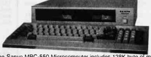
The Sanyo MBC-550 Microcomputer includes 128K byte of memory, a 5 1/4" disk drive along with a parallel printer port. The computer outputs both RGB color and monochrome composite video. Extensive software such as Sanyo Basic, Wordstar, Calcstar and Easy Writer I is included with the MBC-550.
