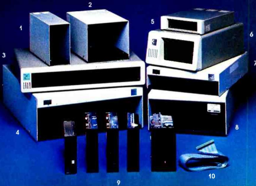
1. **Model # 5SVA&T** - Designed to house one full size or 2 half height 5 1/4" floppy disk drives in the vertical position. As an added feature, the mounting holes are duplicated in reverse so the user can mount the drives door left or door right. The power supply is a custom linear, proven in thousands of installations over the years!
