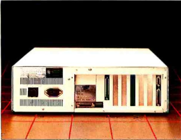
The rear panel of the Leading Edge. Note the serial connector and microswitches in the lower center.
