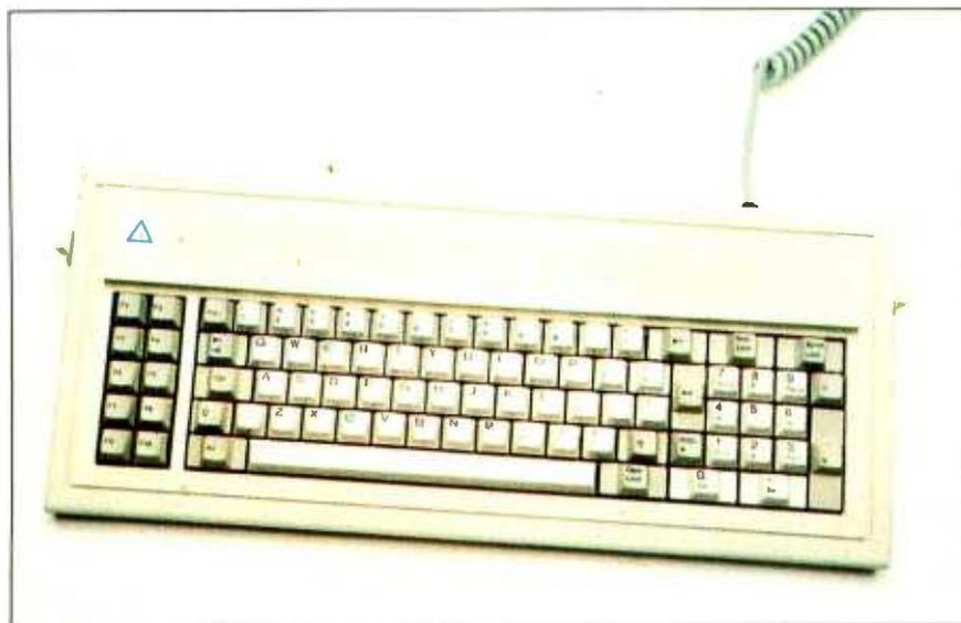
Photo 2: The keyboard of the Leading Edge. Note that the key layout is identical to that of the IBM PC's keyboard.
