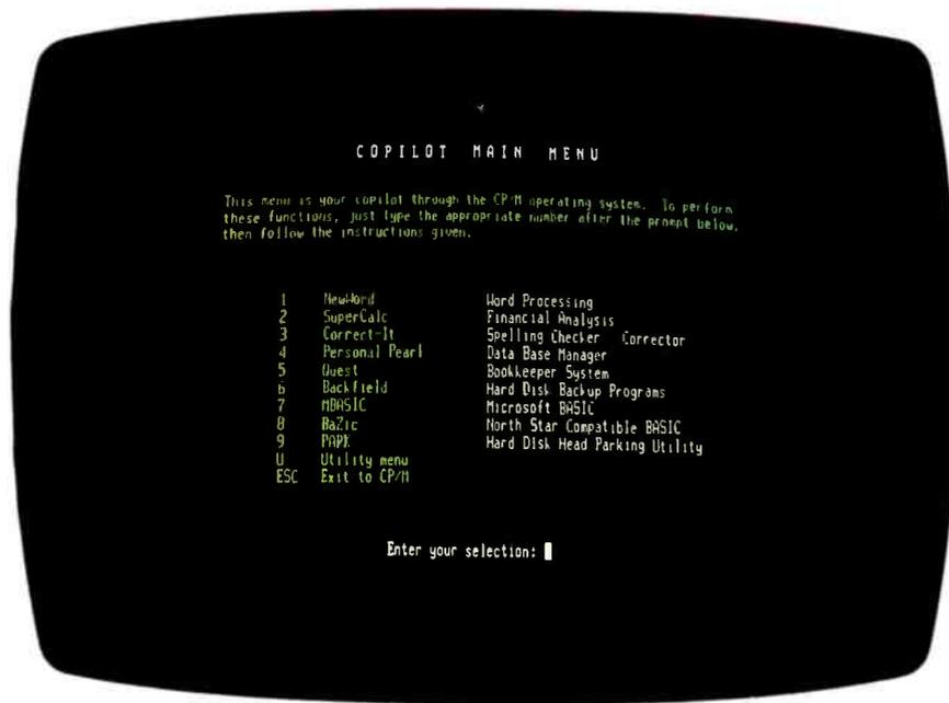
Photo 1: The Co-Pilot menu provides you with access to eight application programs. Additional menu options direct you to PARK (hard-disk heads) and the Utility menu.
