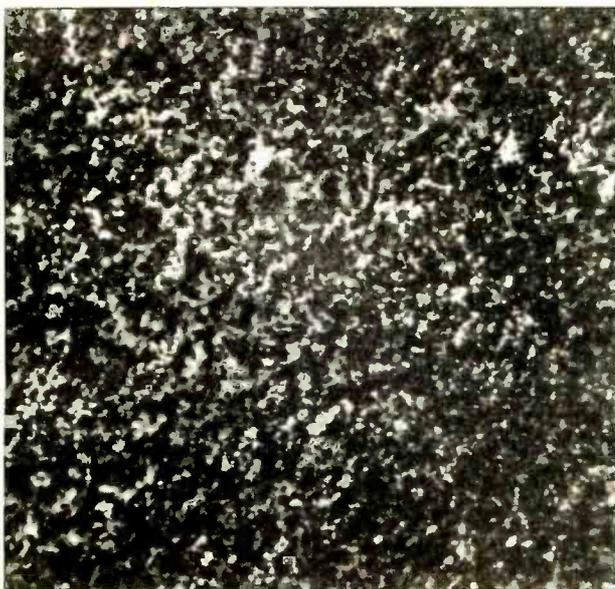
Photo 3: A 128x photograph of a disk typical of the least polished group.
