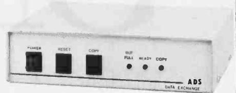
The ADS-8212 DATA EXCHANGE/64K is a computer independent interface converter and print spooler. It can be installed between virtually any computer and any peripheral.
