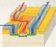
How a transistor operates as a switch.
