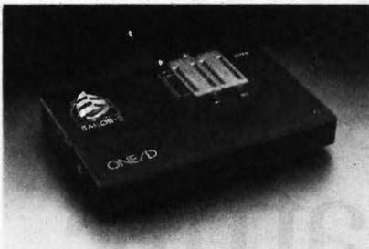
**For economy.** The single-socket SAILOR-1 EPROM programmer is small, portable, and fast. Dual sockets on the SAILOR-2 allow mini-gang and mini-set programming. Macros for totally automated operation!
