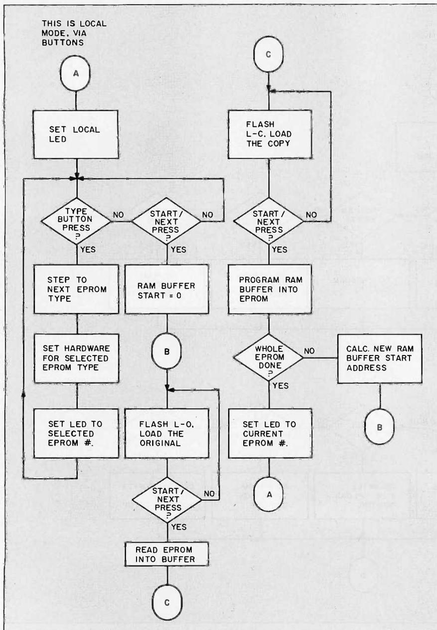
Figure 7c: Flowchart 3, logic flow for the local mode.
