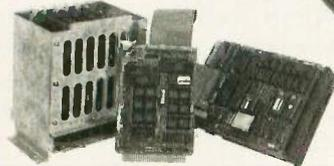
**SCSI/IOP™** - permits connection of off-the-shelf STD bus industrial I/O interfaces (analog, digital, serial, display, power control, etc.)
