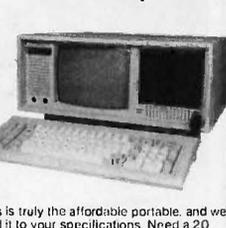
This is truly the affordable portable, and we'll build it to your specifications. Need a 20 meg hard disk and 20 meg tape with 640K memory in your portable? No problem! The **XPC Compact** comes standard with a 9" amber TTL monitor, 135 watt P.S. 256K memory, two 360K drives, Real Time Clock Calendar w/ battery Back-up, serial and parallel ports, and our **TURBO** Motherboard.
