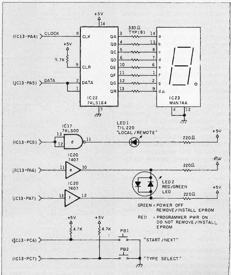
Figure 6: The CCSP's entry/display circuit.
