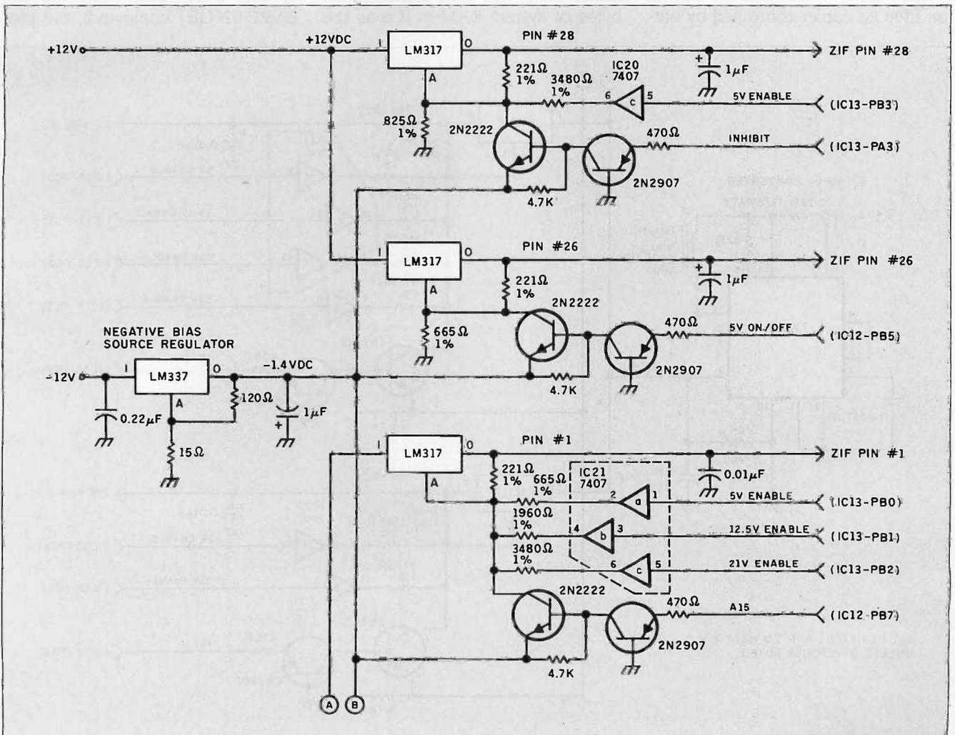
Figure 5: Detailed schematic of the programmer's level-shifting circuitry.
