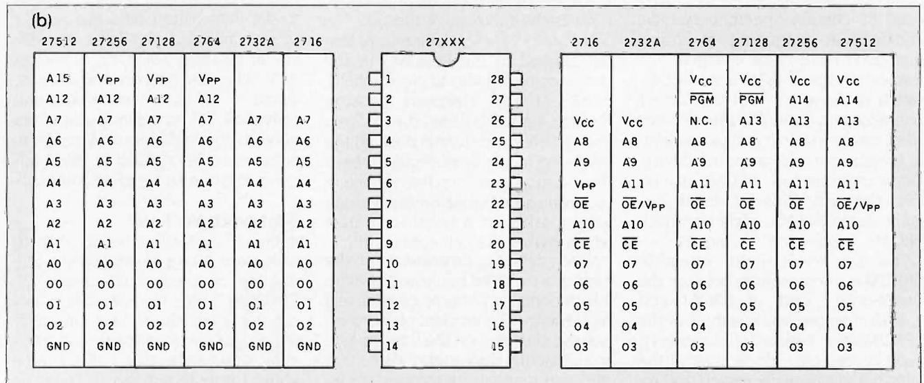
Figure 1: (a) EPROM programming-pin functions by EPROM type. (b) The great EPROM pin-out maze, illustrating the configuration of those EPROMs the CCSP is designed to handle.
