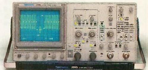
Featuring four channels, flexible triggering, extensive CRT readouts and push-button ease of use, the new Tek 2246 (left) and 2245 (above) bring high-quality, low-cost analysis to diverse applications in digital design, field service and manufacturing.
