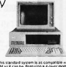
This standard system is as compatible with IBM as it can be. Featuring a 4-layer motherboard, 8-slot expansion, up to 640K memory on the motherboard, and the 6.67 MHz **TURBO** mode. Also included, DOS 3.1, keyboard, 135 watt power supply, TTL 720 x 348 resolution video card, green or amber monitor, serial & parallel ports. Real Time Clock and software.
